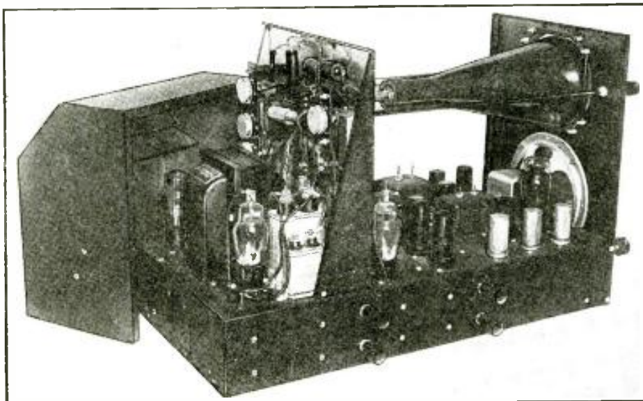
A close-up view of the 5-in. telly receiver with rear safety cover removed. The 2 upper controls on the side skirt are for image size and the lower 2 are for vertical and horizontal speed control.
