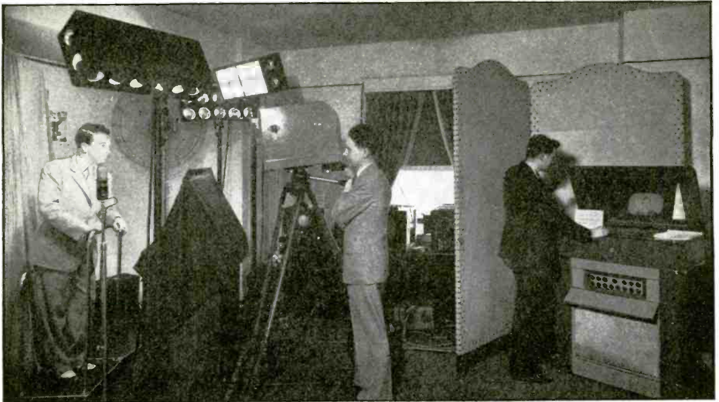
Scene in temporary television studios in first 2-way 441-line wire-television demonstration. "Jeep" control at right.
